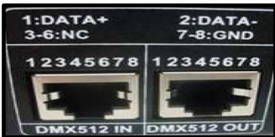
Uses RJ45 as interface signal
