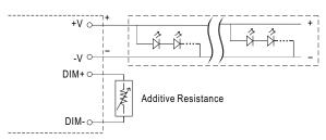
"DO NOT connect "DIM- to -V"
