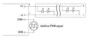
"DO NOT connect "DIM- to -V"
