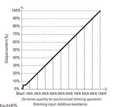
Note: 1. Min. dimming level is about 6% and the output current is not defined when 0%< Iout<6% 2. The output current could drop down to 0% when dimming input is about 0kΩ or 0Vdc, or 10V PWM signal with 0% duty cycle.
